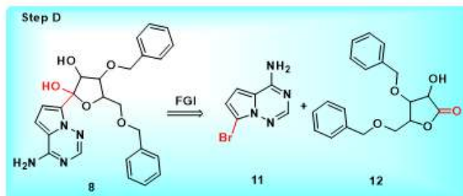
Figure 6: General mechanism of Alcohol synthesis, Disconnection of compound 8 (alcohol) to compound 11 (aryl halide) and compound 12 (ketone).
